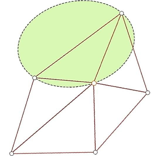
Build a mesh s.t. **the star of each vertex is Delaunay**
